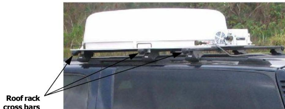
**Figure 2-4. Roof Rack Mounting**
