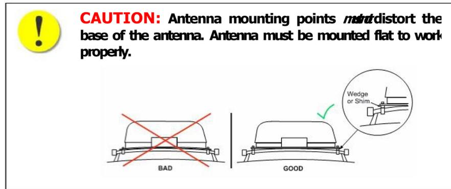
**To install the antenna to a vehicle roof rack**
