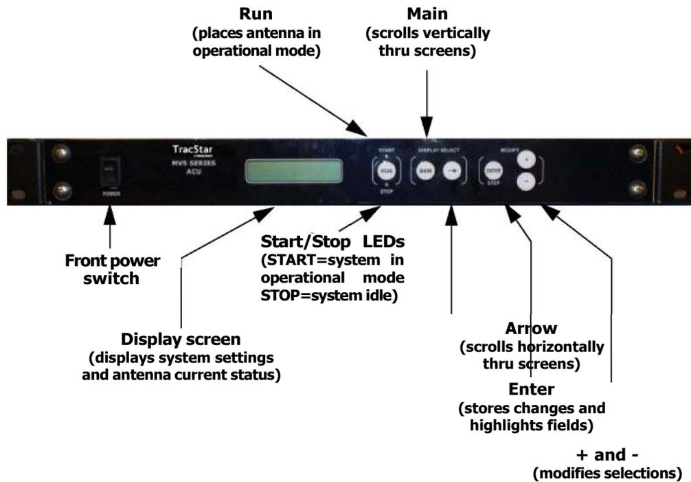
Figure 5-1. TracStar i450M ACU Control Panel
