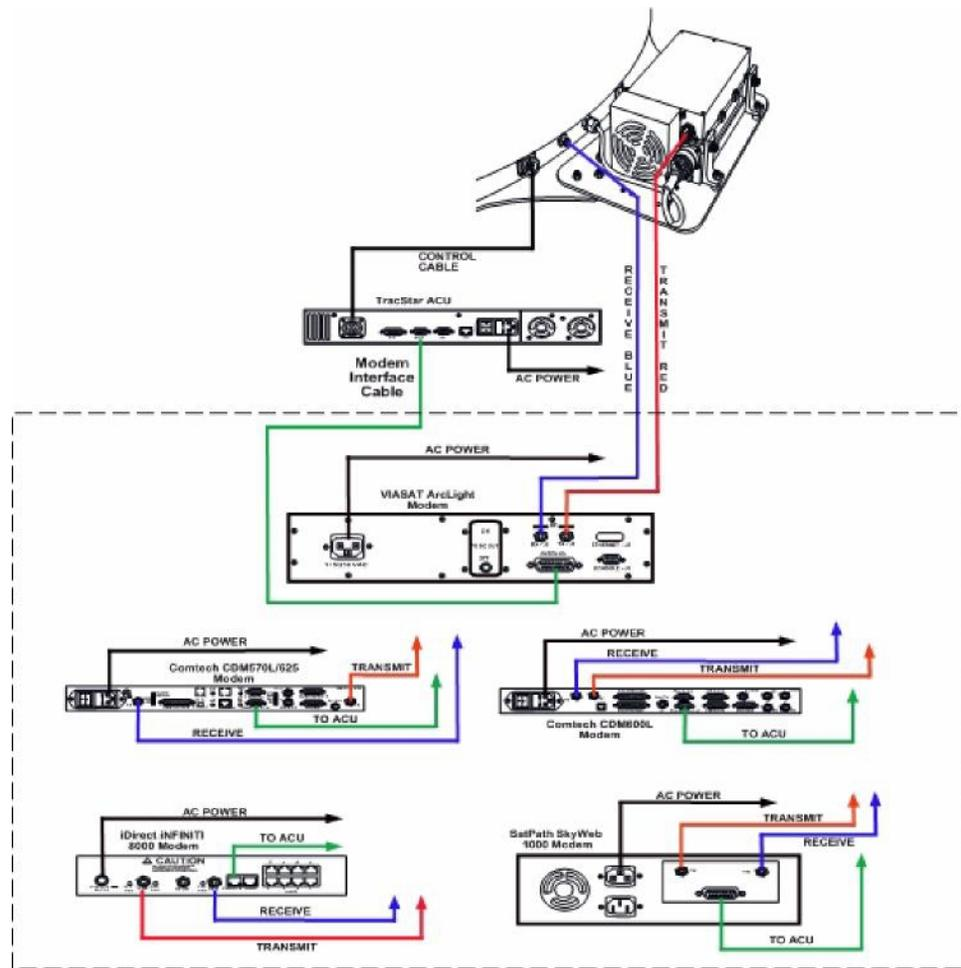
Figure 2-11. ACU and Modem Cable Connections – Supported Modem Types
