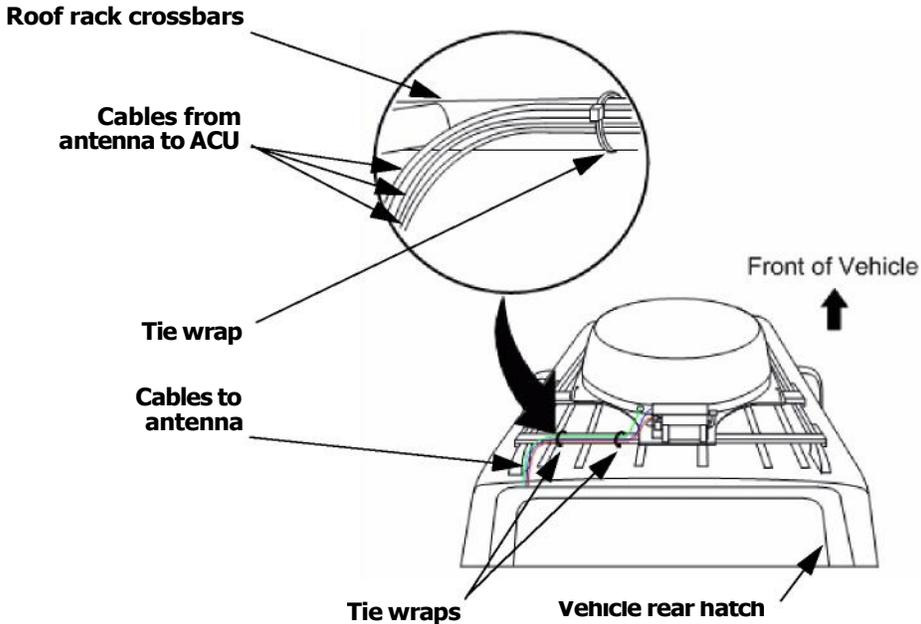
Figure 2-9. Securing Cables to the Roof Rack with Tie Wraps
