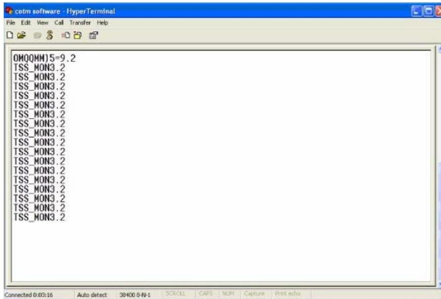
**Figure C-4. HyperTerminal Window – Boot Process Stopped**
