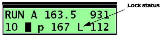
Figure 3-3. Run Screen: Locked
