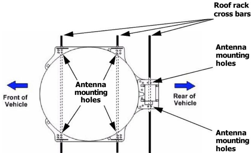
Figure 2-5. Antenna-to-Rack Positioning
