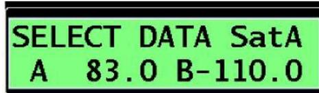
Figure 4-13. Select Data Screen – Data Satellite Orbital Location Example
