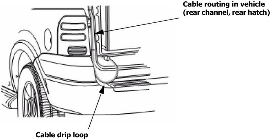
Figure 2-10. Cable Drip Loop
